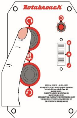
3) Motor OFF Press the top button on the control panel again. Once pressed the green illumination will no longer light up, this means the motor has stopped.
